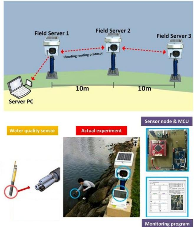
Fig. 2: Test-bed architecture and practical experiment.
