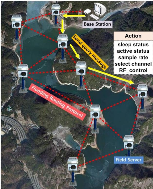
Fig. 1: Concept of water quality monitoring system.
